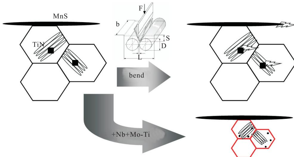
**Fig.12.** Schematic illustration of the mechanism of improving bending property.
