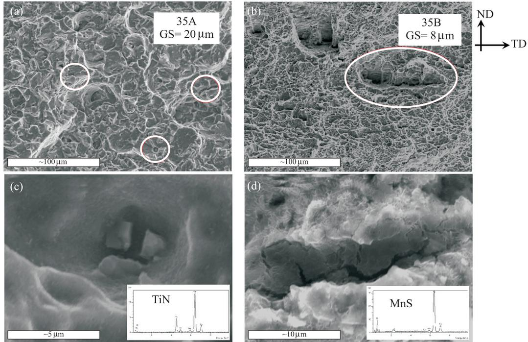
**Fig.11.** Fracture morphology of hot stamped steels after the bending test, (a) 35A, (b) 35B, (c) EDS analysis of TiN, (d) EDS analysis of MnS.
